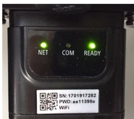
Figure 63 - Irregular communication status between inverter and adapter
