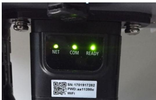
Figure 62 - Final status of LEDs
