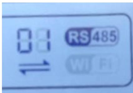
Figure 82 - RS485 symbol on the display of the inverter
