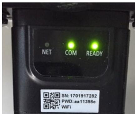
Figure 64 - Irregular communication status between the adapter and remote server
