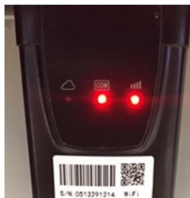
Figure 43 - Initial status of LEDs
