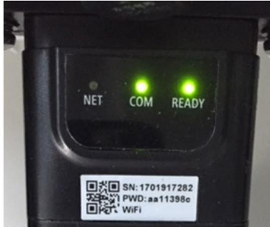
Figure 58 - Irregular communication status between the adapter and remote server
