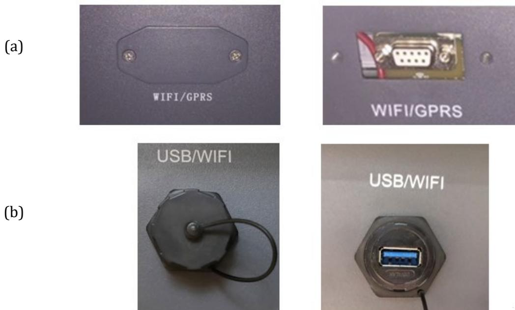
Figure 26 – Port for external Wi-Fi adapter
