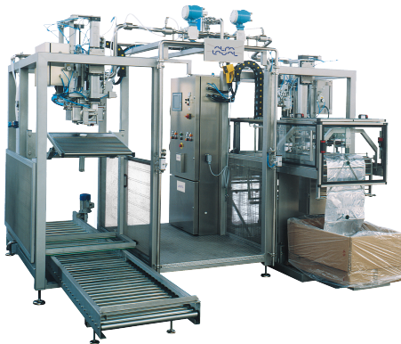
CAF filler with 3–20 litre (1–6 gallons) automatic bag feeder (right head) and mobile roller conveyor (left head).
