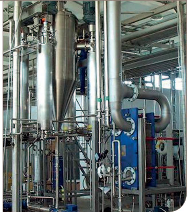
Quadruple Contherm/Convap installation with plate heat exchanger as condenser.
