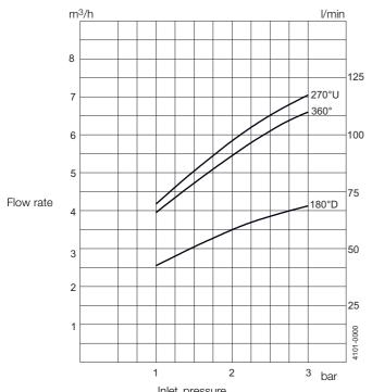
Inlet pressure For clip-on models, the flow rate is increased by approx. 0.5  $\,\mathrm{m}^3/\mathrm{h}.$
