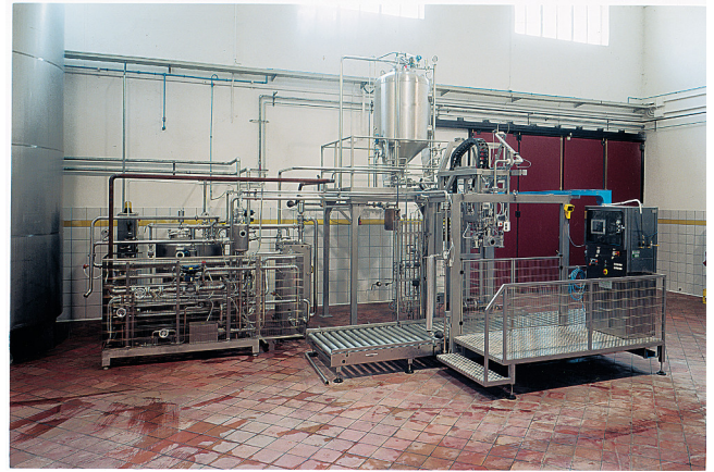
Alfa Laval Steritherm plate sterilizer PHE 5000 with a 1000 litre (300 gallons) aseptic tank and TAF filler 1 HM/1 inch.
