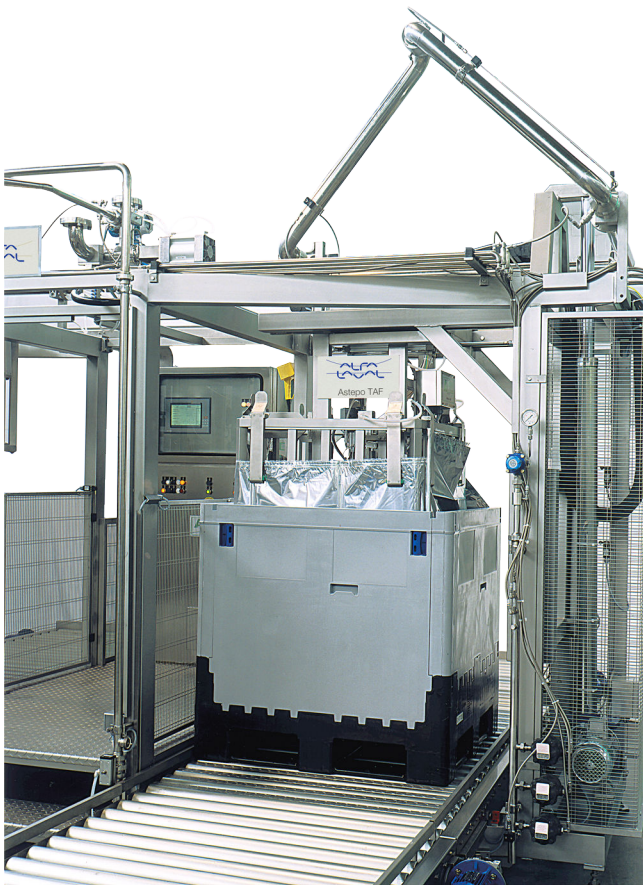
Filling of a 1000 litre (300 gallons) container.
