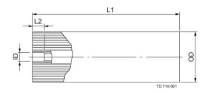
OD = outer diameter of spiral membrane
