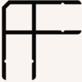
SİDİNG KENAR KAPAMA ( SIDING EDGE CLOSURE )
