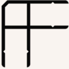
SIDING KENAR KAPAMA ( SIDING EDGE CLOSURE )
