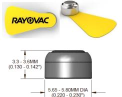
DIMENSIONS SHOWN ARE IEC STANDARDS. FOR ENGINEERING TOLERANCES CONTACT RAYOVAC.
