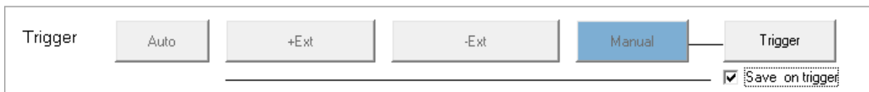
Trigger selection radio button on main panel (PicoVNA 108) Note that Save on Trigger works in +Ext, -Ext and Manual modes only.
