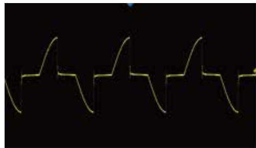
TrailingEdge phase dimming
