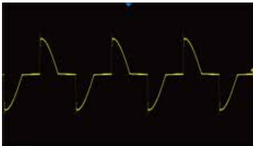
LeadingEdge phase dimming
