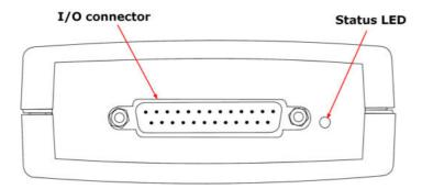
**I/O connector:** for the pin-numbering of the I/O connector, see <u>I/O connector pins</u>. The Pico PP545 Small Terminal Board is specially designed to connect to this socket to allow you to make connections to individual wires easily without soldering. If you need to use a ribbon cable to connect your signals to this socket, use the shortest possible length to avoid introducing too much crosstalk between the signals.
