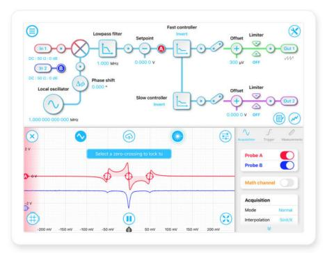
Demod. Frequency 1 mHz to 200 MHz Scan Frequency up to 1 MHz Adjustable Filter DAC Res 1 kHz to 14 MHz 16 Bits Built-in Control Dual PID Integrated Oscilloscop 500 MSa/s
