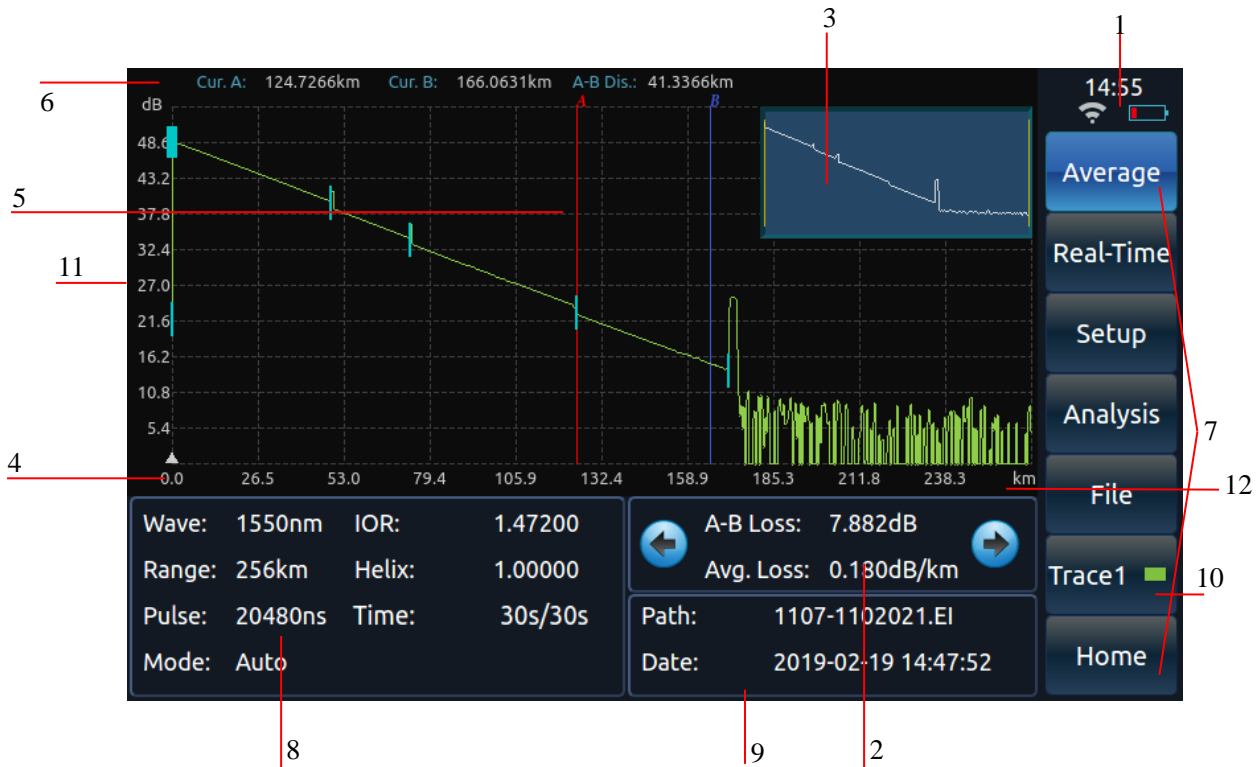
Fig. 3-1 Diagram of 6422 OTDR testing interface
