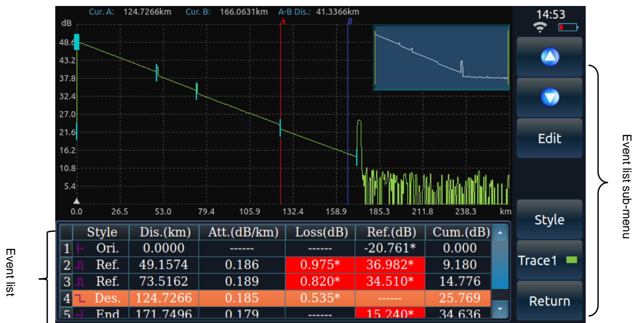
Fig. 3-2 Diagram of 6422 OTDR analysis interface
