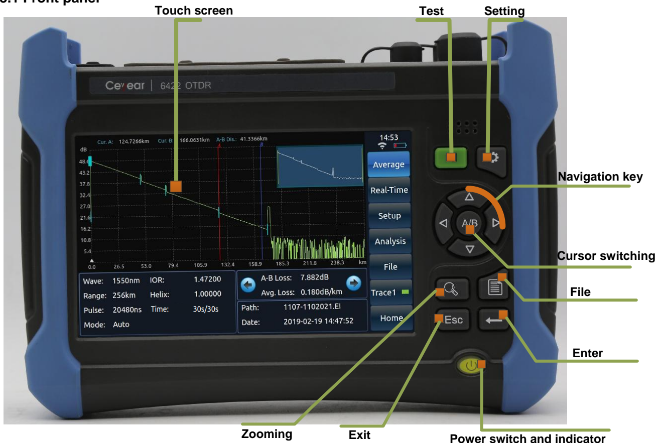
Fig.1-1 Front panel of the 6422 optical time-domain Reflectometer
