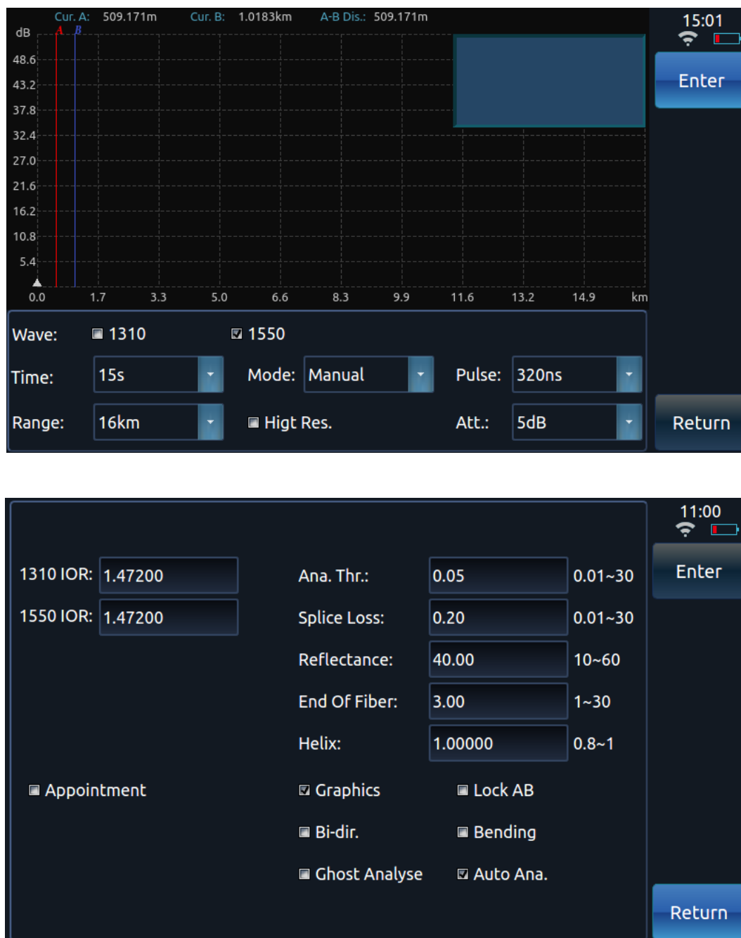
Fig. 3-5 Window of setting 6422 OTDR test conditions
