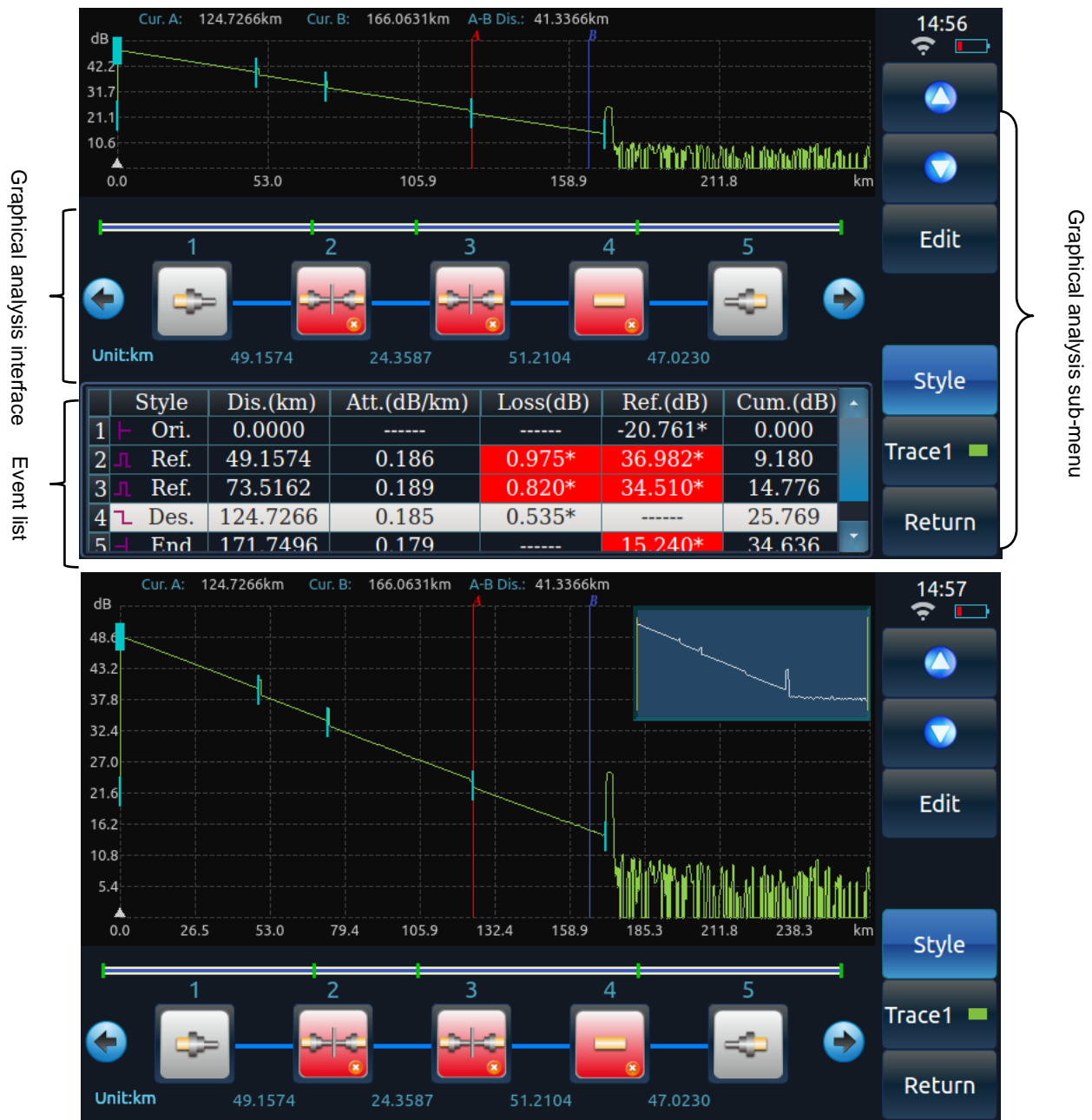
Fig. 3-3 Diagram of 6422 OTDR graphical analysis interface
