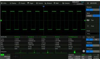
Statistics show the current value, maximum value, minimum value, standard deviation, and mean value of up to 12 parameters simultaneously. A histogram is available to show the probability distribution of a parameter. Trend and Track are available to show the parameter value vs. time.
