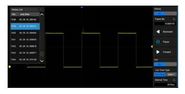
History function can record up to 80,000 frames of waveforms. The recording is executed automatically so that the customer can playback the history waveforms at any time to observe unusual events and quickly locate the area of interest using the cursors or measurements. The failed frames of the Mask Test can be stored as history
