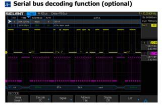
SDS1000X/SDS1000X+ displays the decoding through the events list. Bus protocol information can be quickly and intuitively displayed in table form.
