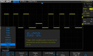
SDS1000X/SDS1000X+ has a wealth of trigger modes, including Edge, Slope, Pulse, Video, Windows, Runt, Interval, Time out (Dropout), Pattern, IIC, SPI, UART/RS232, LIN, CAN
