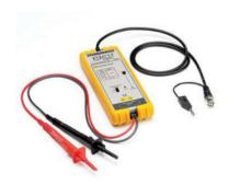
The TA041 is an active differential probe suitable for high common-mode voltage measurement applications up to  $\pm 700~V~$  (DC + peak AC). It can be used with signal speeds of up to 25 MHz.
