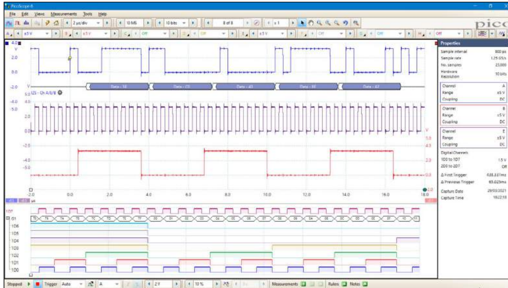
Analog waveforms (top) and digital waveforms (bottom) shown on PicoScope 6 display
