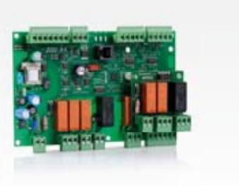
**10 inputs/9 outputs control module**
