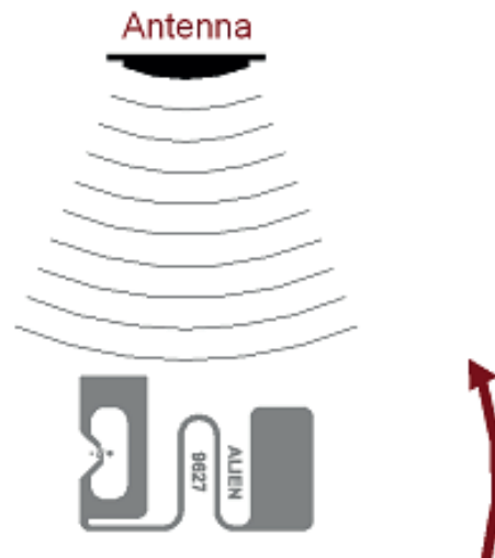
Angular Sensitivity Inlay is rotated in the x, y, plane about the z axis
