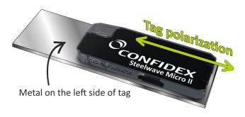
When mounting the tag with its adhesive background, clean and dry the surface for obtaining the maximum bond strength.
