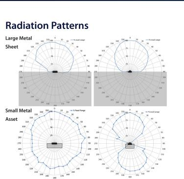
Radiation patterns for the embedded version will vary dependent on the geometry and composition of the asset type.
