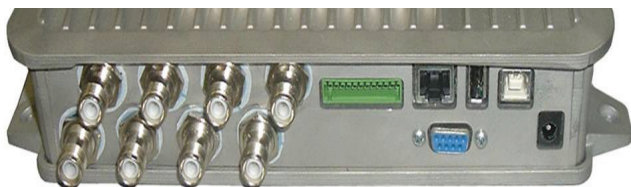
Figure 1-2 FX9500 Power and I/O Connections
