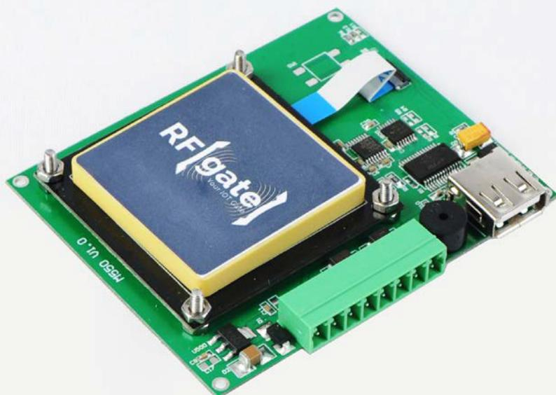
FPC Connector (8Pin , spaces between PINs: 0.5mm)
