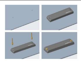
Instructions for optimal performances: 1.Drill two holes on the subject metal surface. (ø 4.0 mm), pitch: 65.7mm) 2.Insert two  $\phi 3.4 mm$  (recommended size) rivets on the tag. 3.Fix the tag on the metal surface with a rivet gun.
