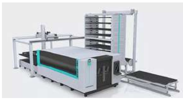
Automatic Loading And Unloading System
