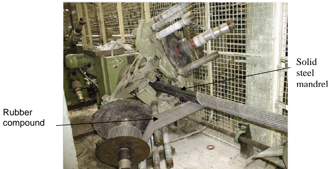
Figure 3.2 Shows tube compound being wrapped on to a mandrel
