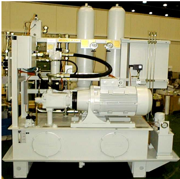
Figure 3.3 – An industrial power unit with large well-spaced reservoir Note the inspection covers on the front of the unit allowing cleaning and inspection of internals
