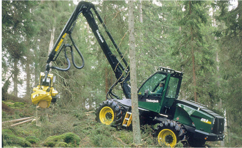
Figure 3.1 showing the diverse working angles of a mobile machine, which entails good reservoir design and internal layout
