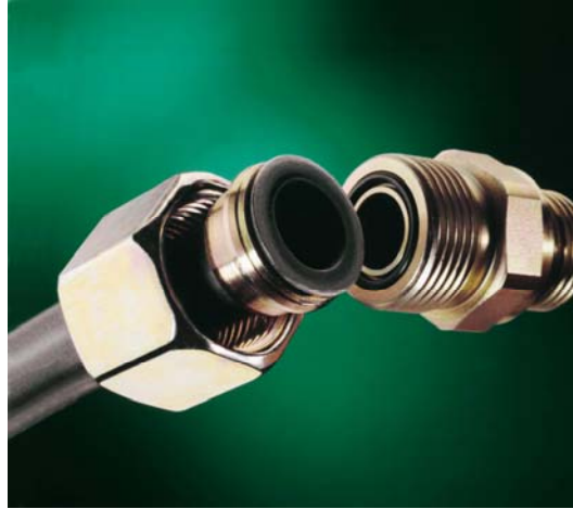
Figure 3.5.1.2 – ( Parker Hannifin ) O-Lok– Mechanical tube end preparation in the form of a flat face flange enables the tube to sit squarely against the face of the fitting seal enabling positive assembly and a ‘soft seal’ leak free connection
