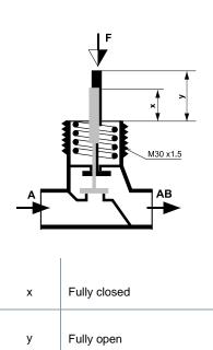
Thermal actuator 6.5 mm stroke with ASA80 adapter
