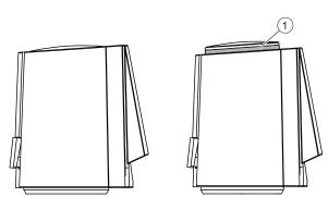
The movement and position of the actuator valve is indicated by the stroke indicator (1).
