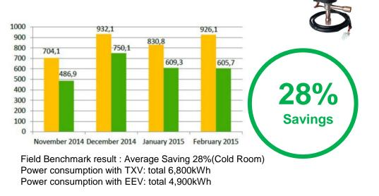
Fast pull down : better exchange in the evaporator Stable Superheat whatever the external conditions (1K=3% COP) Stable Evap Temp : avoid low temp and defrost cycle
