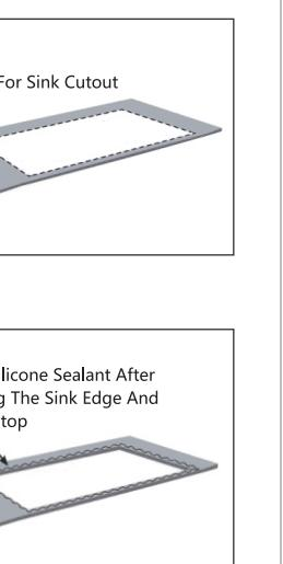
1. Position the cut-out template front to rear so the sink will not interfere with the cabinet; secure with tape.
