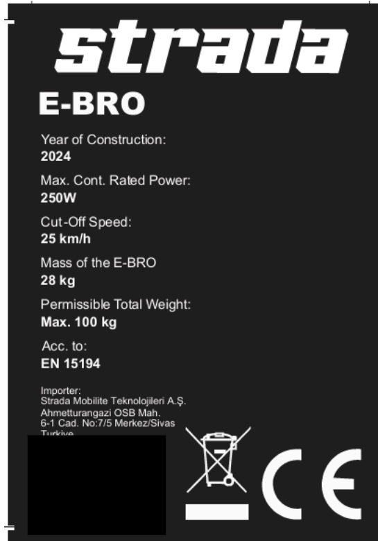
Figure 2 The Photo of nameplate
