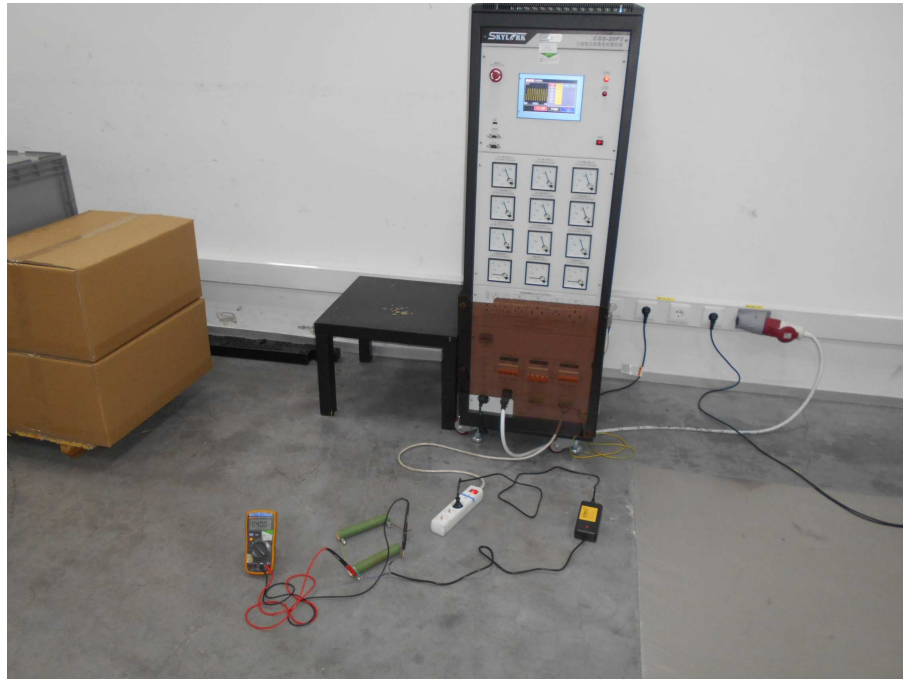
Photograph 6: Set-up for immunity test of voltage dips
