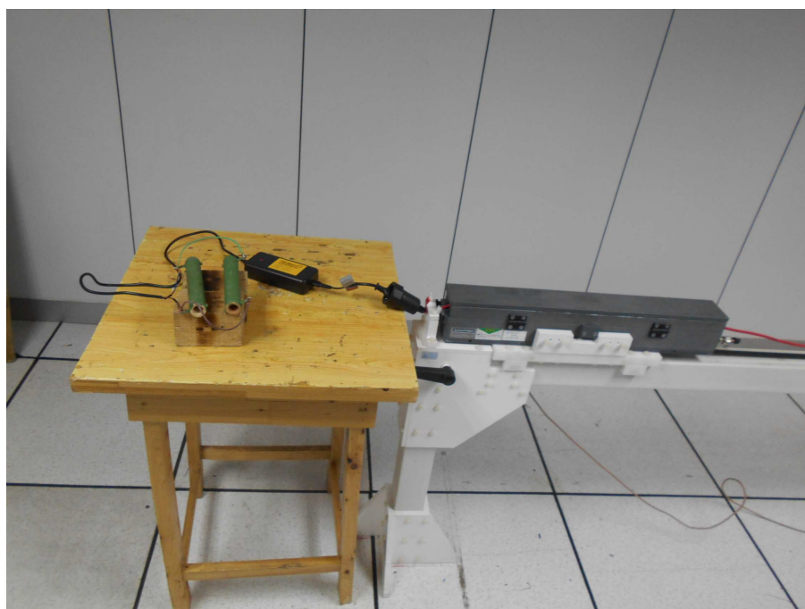
Photograph 2: Set-up for measurement of disturbance power
