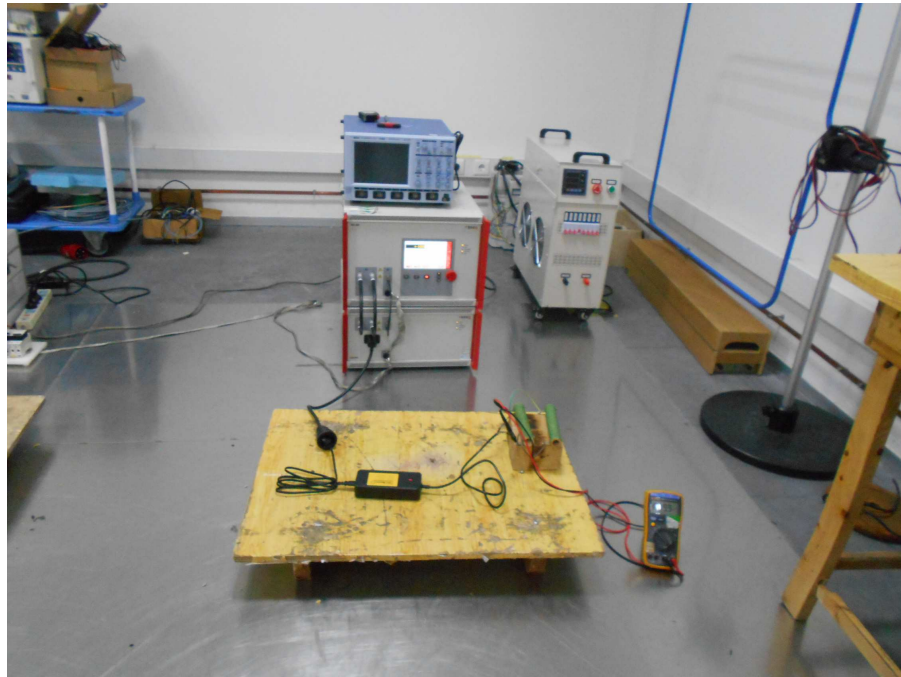
Photograph 5: Set-up for immunity test of injected current
