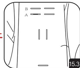
When using the sleeping mode, the restraint system shall be removed. When removing the restraint system, you can directly take out the ladder lock buckle at the end of the seat belt under the backplane. When installing the seat belt, the ladder lock buckle at the end of the seat belt should be stuck under the backplane. When use seating mode, the restraint system must be used.
