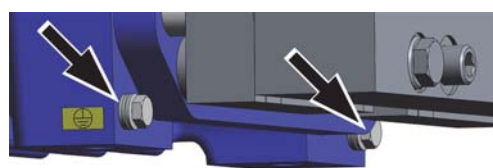
Figure 5-3-6-02 - Protective earth connection
