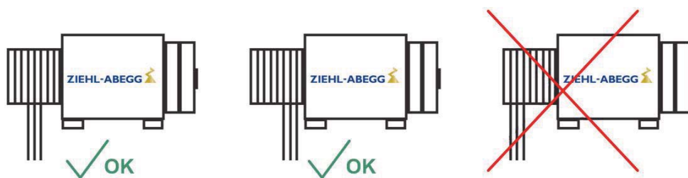
Figure 4-3-01 - Fitting the ropes
