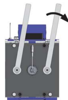
Figure 6-5-2-03 Brake manuell released Example for hand release lever position
