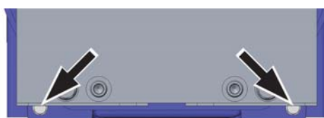
Figure 5-3-6-01 - Protective earth connection
