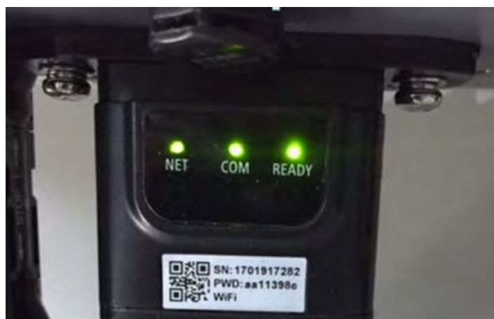
Figure 72 - Final status of LEDs
