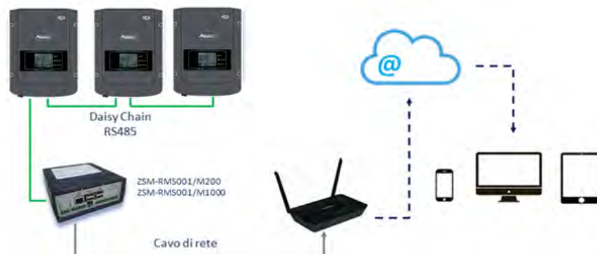
Figure 82 – Diagram showing the operation of the ZSM-RMS001/M200 / ZSM-RMS001/M1000 datalogger
