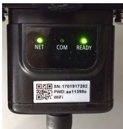
Figure 62 - Irregular communication status between inverter and Wi-Fi
