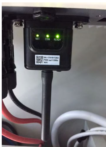
Figure 60 - Final status of LEDs
