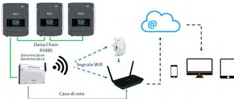
Figure 81 – Diagram for connecting the ZSM-DATALOG-04 / ZSM-DATALOG-10 datalogger
