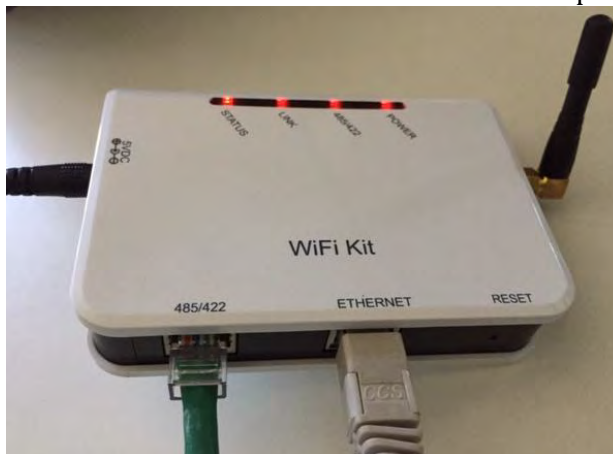
Figure 89 – Ethernet cable connected to the datalogger
