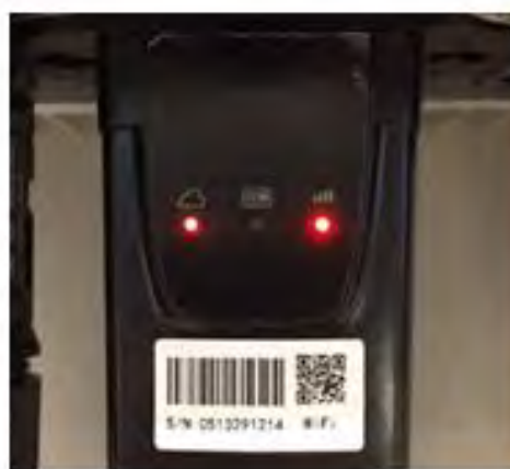
Figure 62 - Irregular communication status between inverter and Wi-Fi
