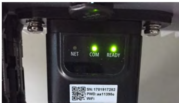
Figure 77 - Initial status of LEDs
