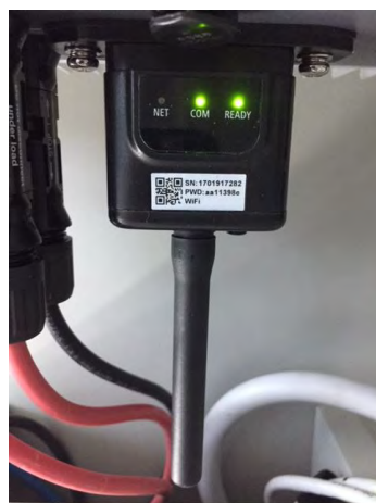
Figure 59 - Initial status of LEDs
