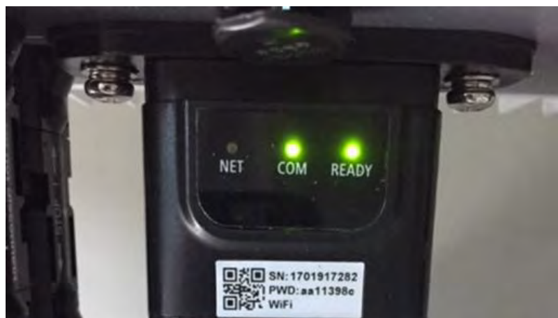
Figure 71 - Initial status of LEDs
