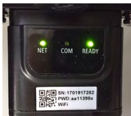
Figure 79 - Irregular communication status between inverter and adapter
