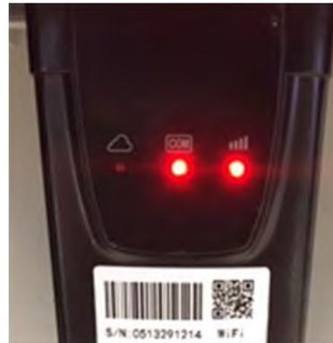
Figure 59 - Initial status of LEDs
