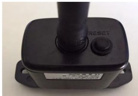
**Figure 61 – Reset button on the Wi-Fi adapter**
