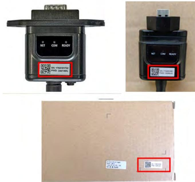
Figure 47 - Password of external Wi-Fi adapter
