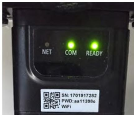
Figure 80 - Irregular communication status between the adapter and remote server
