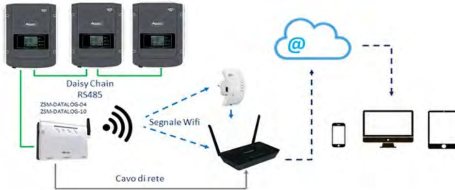
Figure 81 – Diagram for connecting the ZSM-DATALOG-04 / ZSM-DATALOG-10 datalogger
