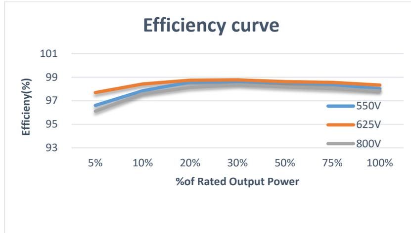
Figure 10 - Power efficiency curve (take 80KW for example)
