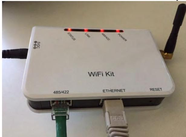
Figure 89 – Ethernet cable connected to the datalogger
