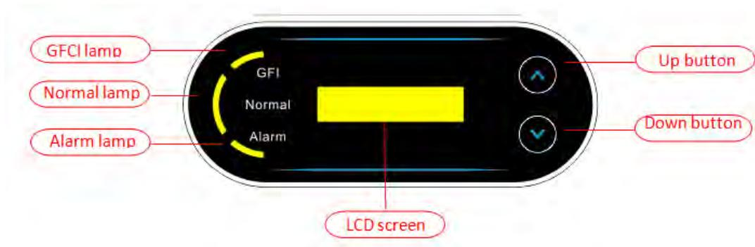
Figure 38 - LCD display with buttons and LED indicators
