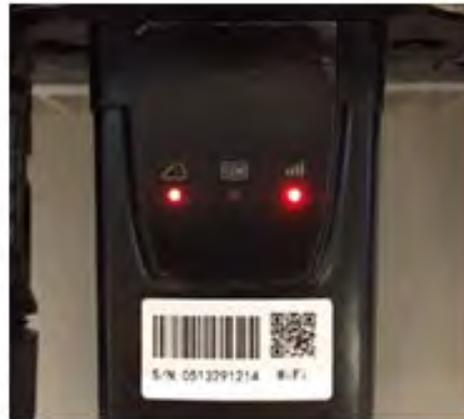
Figure 62 - Irregular communication status between inverter and Wi-Fi
