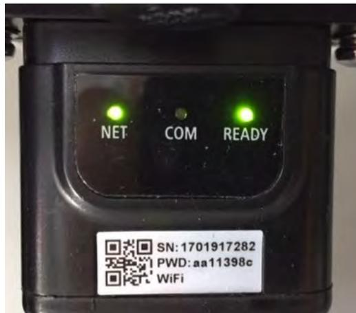
Figure 73 - Irregular communication status between the inverter and adapter
