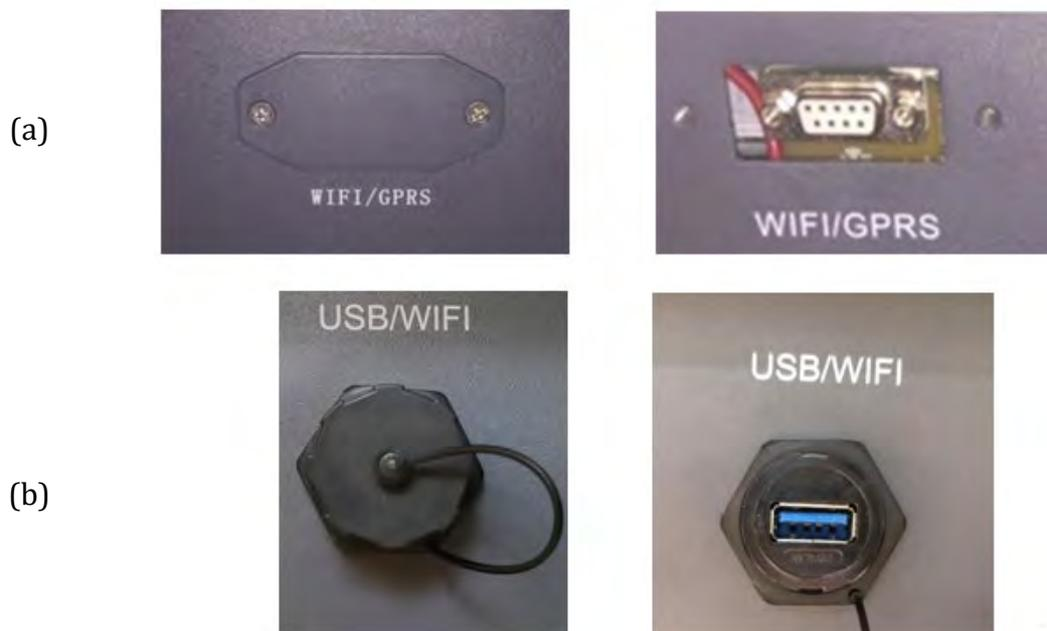
Figure 42 – Port for external Wi-Fi adapter
