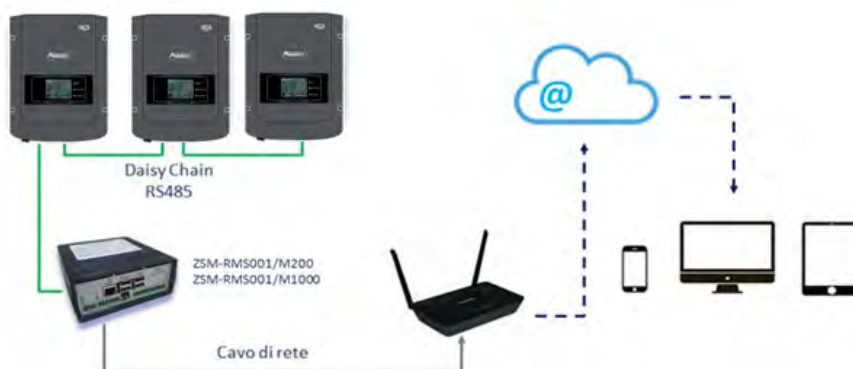
Figure 253 – Diagram for the functioning of the ZSM-RMS001/ M200 / ZSM-RMS001/M1000 datalogger
