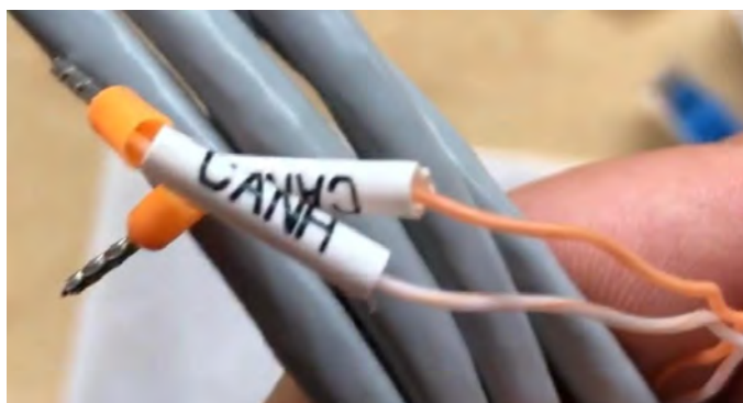
Figure 93 - Inverter/HV BOX communication cable
