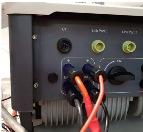
Figure 101 - Inverter-side DC power connection with two battery inputs populated
