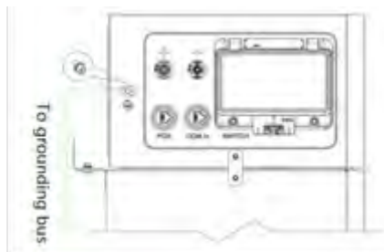
Figure 152 - Connection of grounding cable
