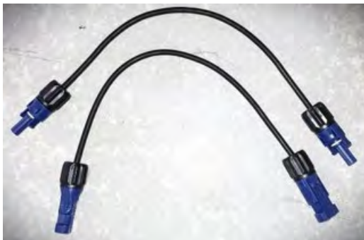
Figure 124 - Power connector between battery modules
