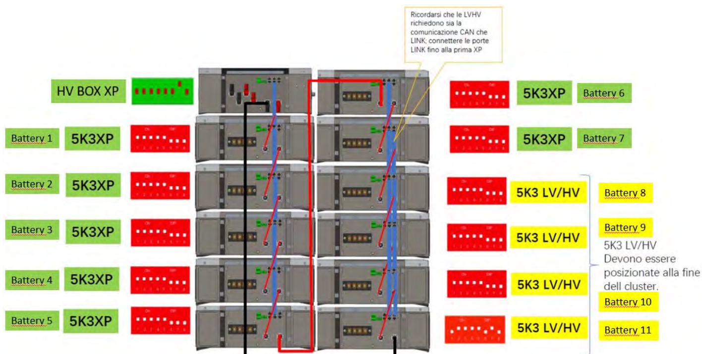
Figure 112 - Power connection and 5K3 and 5K3XP battery communication
