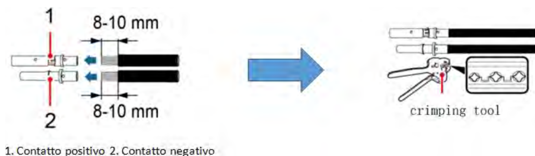
Figure 20 – Preparing the positive and negative photovoltaic cables
