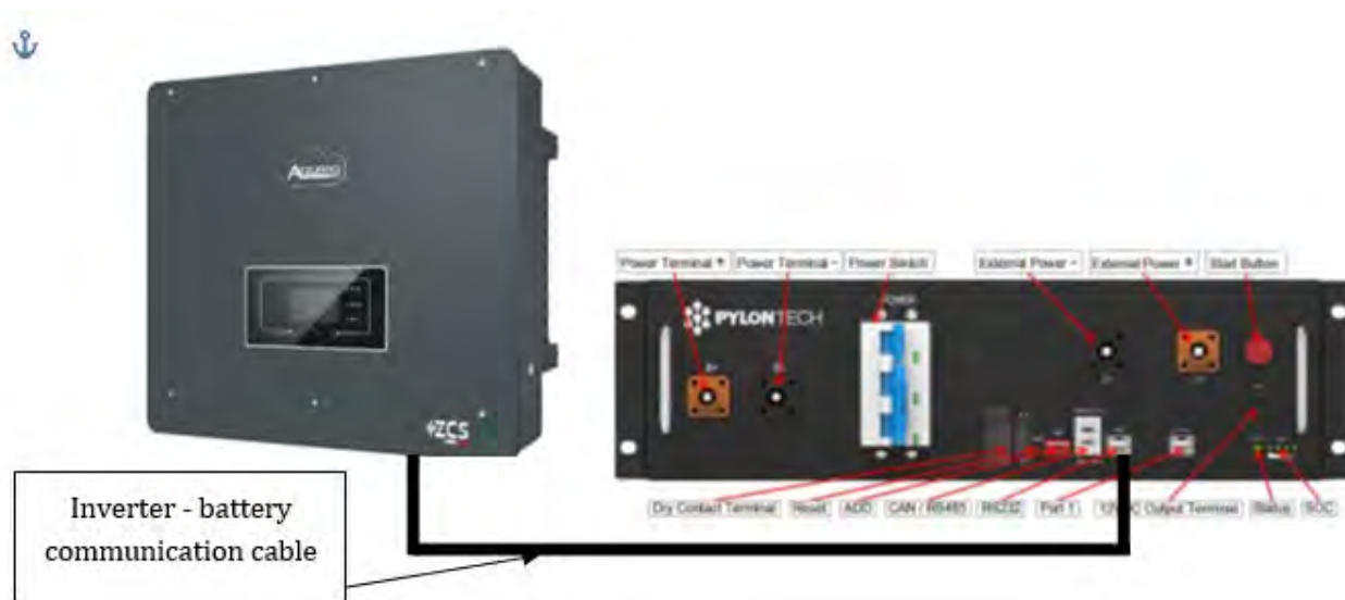
Figure 32 - Hybrid inverter and BMS communication connection
