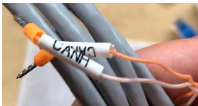
Figure 70 - Inverter/HV BOX communication cable
