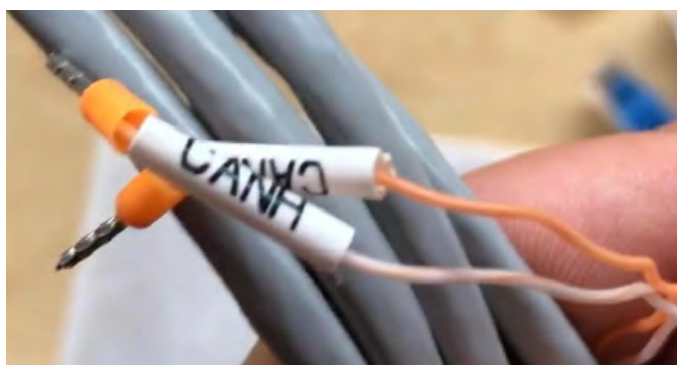
Figure 105 - Inverter/HV BOX communication cable
