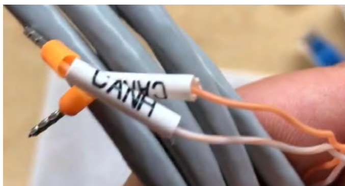
Figure 81 - Inverter/HV BOX communication cable
