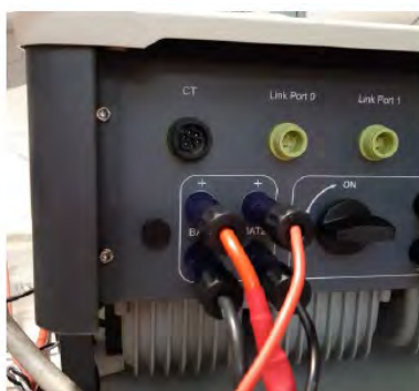
Figure 183 - Power connection DC inverter side with double battery input populated
