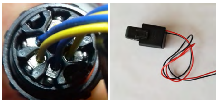
Figure 190 - Numbered connections of the CT connector
