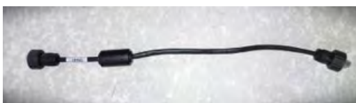
Figure 172 – Communication cable between BDU Smart 5K 1 and BDU
