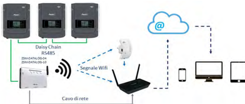
Figure 252 – Diagram for connecting the ZSM-DATALOG-04 / ZSM-DATALOG-10 datalogger
