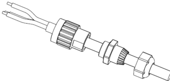
Figure 19 - Connecting the AC output cables (2)
