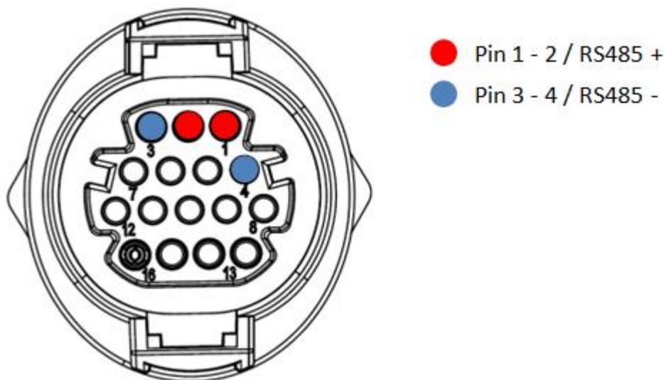
Figure 98a – Connecting the serial line via the communication connector for 3PH HYD5000-HYD20000-ZSS
