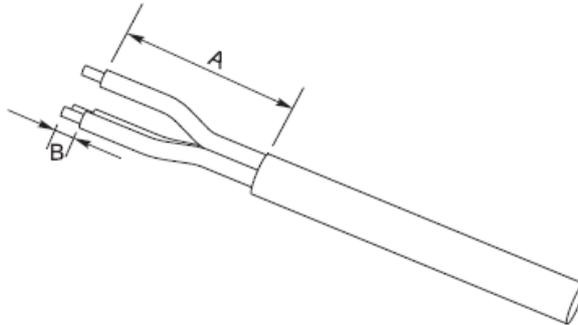
Figure 18 - Connecting the AC output cables (1)
