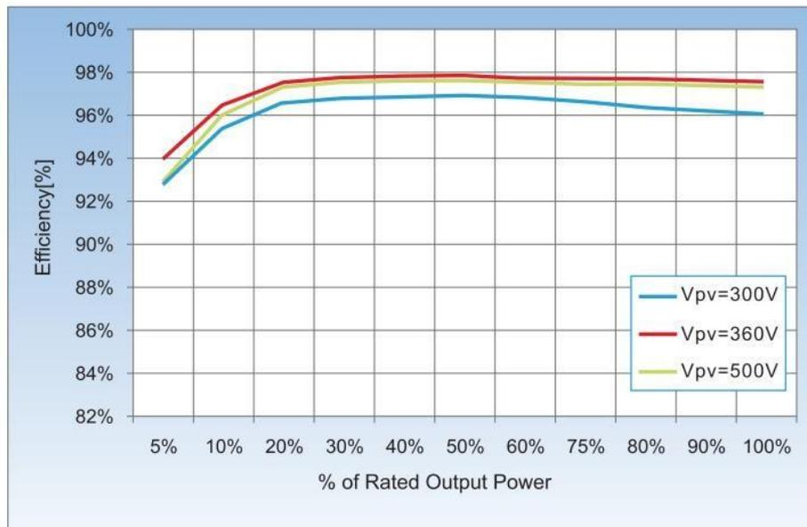
Figure 7 - Power efficiency curve
