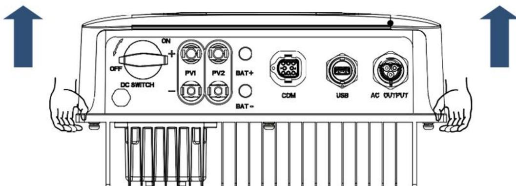
Figure 6 - Removing the inverter from its packaging
