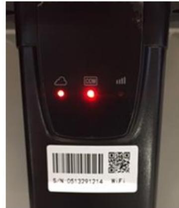
**Figure 56 - Final status of LEDs**
