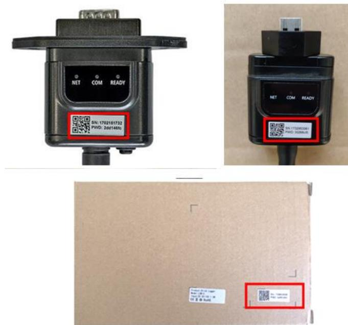
Figure 43 – Password of external Wi-Fi adapter
