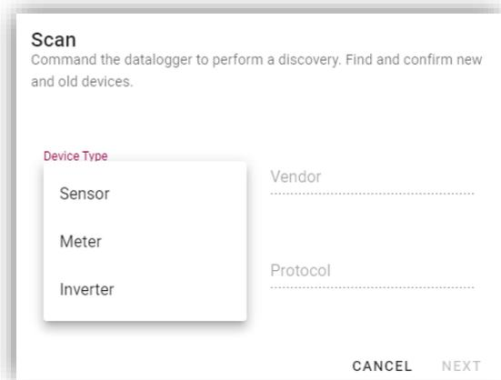
If a meter is one of the devices connected to the Datalogger, select the type of Meter/Datalogger communication interface and the relative communication protocol.
