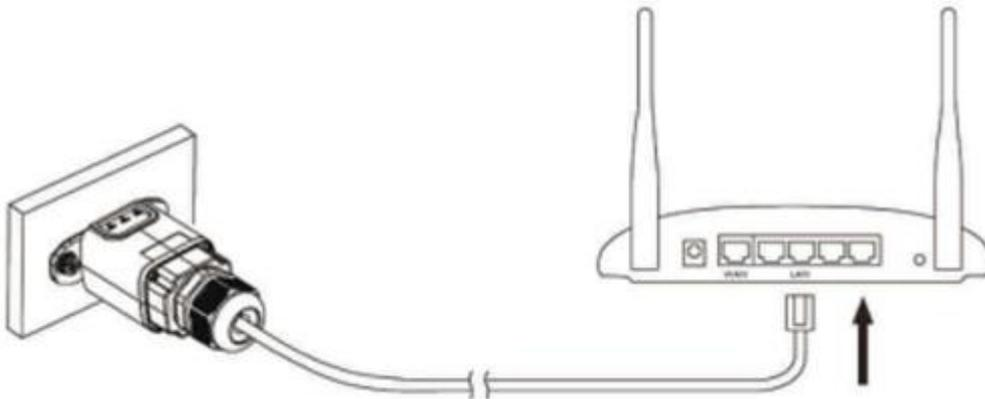
Figure 66 - Connecting the network cable to the modem
