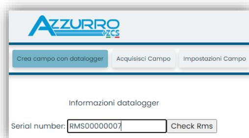
Enter the serial number (S/N) of the datalogger and click “Check RMS”. If the datalogger has been configured correctly, a screen will open where you can enter the required information relating to the field to be installed.
