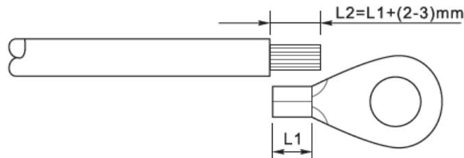
Figure 9 - Preparing the ground cable (1)
