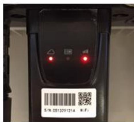
Figure 58 - Irregular communication status between inverter and Wi-Fi
