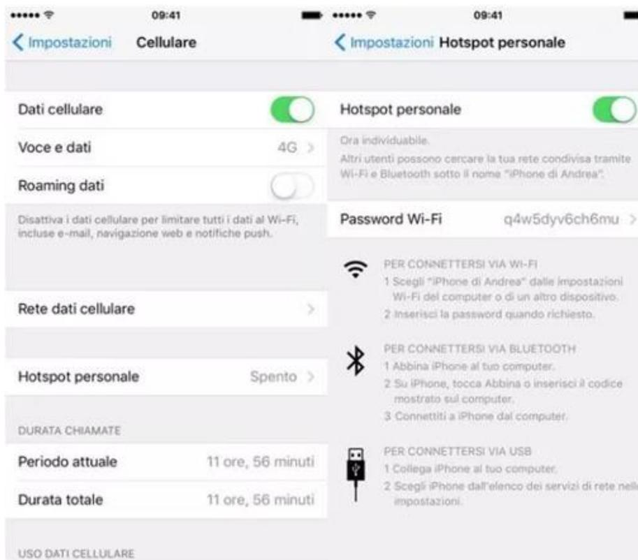
Figure 62 - Configuration of an iOS smartphone as a hotspot router
