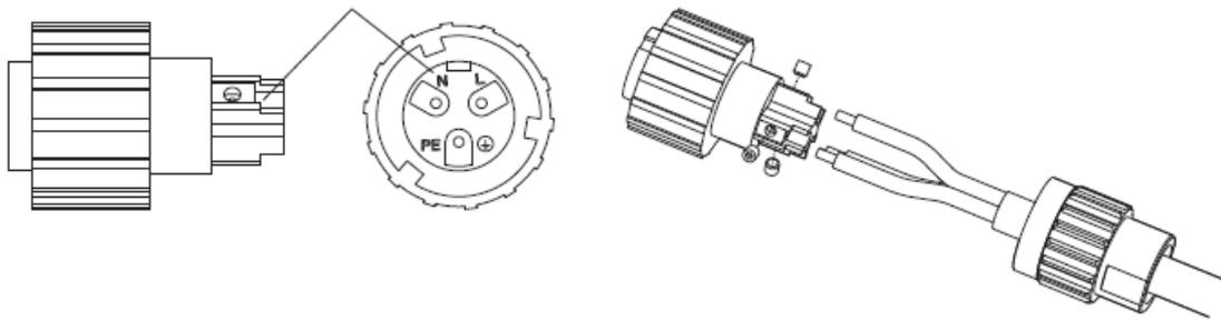
Figure 20 - Connecting the AC output cables (3)
