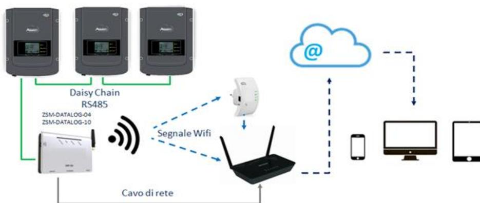
Figure 77 – Diagram for connecting the ZSM-DATALOG-04 / ZSM-DATALOG-10 datalogger
