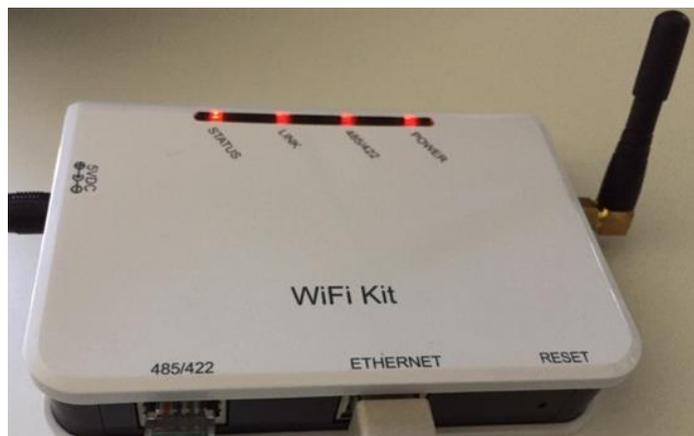
Figure 98 – LED indicating the correct configuration of the datalogger
