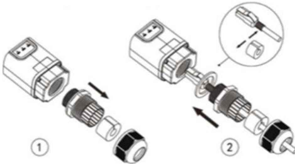
Figure 64 - Inserting the network cable inside the device
