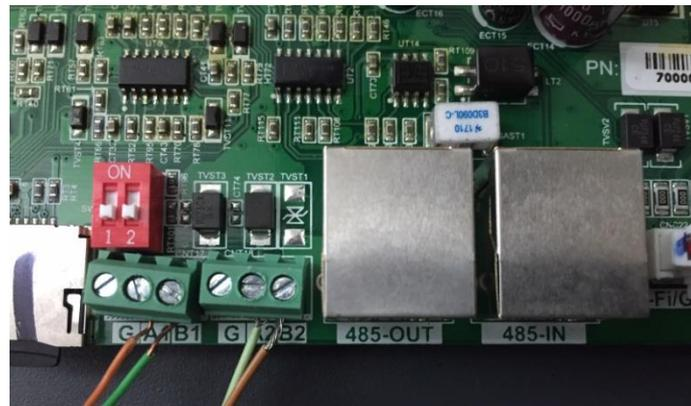
Figure 81 - Connecting the serial line via the RS485 terminal block and via the RJ45 plug
