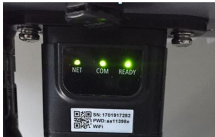
Figure 68 - Final status of LEDs
