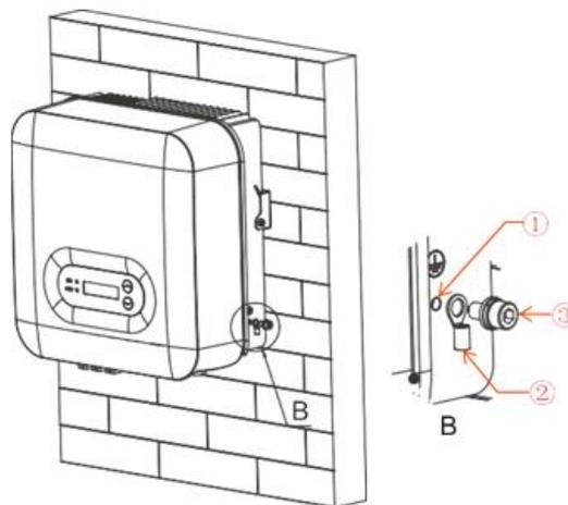
Figure 18 - Inverter external grounding instruction diagram
