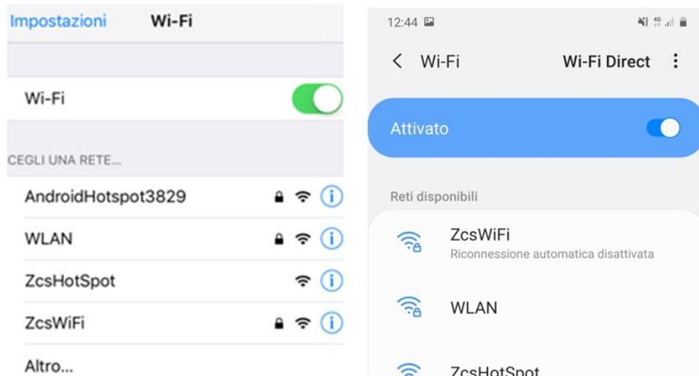
**Figure 53 – Wi-Fi network search on Smartphone (iOS and Android); Access point of the Wi-Fi adapter is no longer visible**
