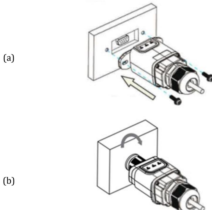
Figure 65 - Inserting and securing the ethernet adapter
