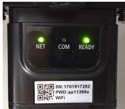
Figure 75 - Irregular communication status between inverter and adapter
