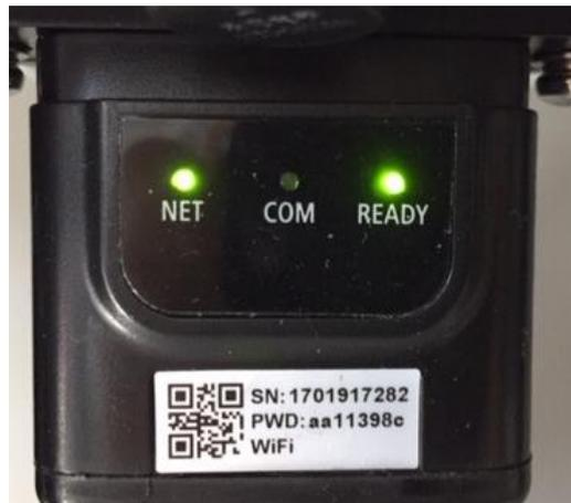
Figure 69 - Irregular communication status between the inverter and adapter
