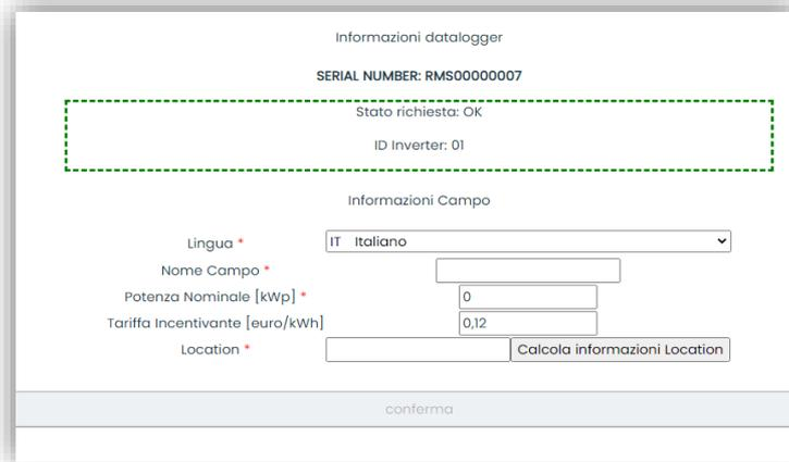
Once the “location” of the field has been entered, click “Calculate Location Information” to allow the system to obtain the latitude, longitude and time zone of the installation. Click “Confirm” to complete the configuration of the field. You only need to wait a few minutes to view the data flow on the ZCS Azzurro portal.
