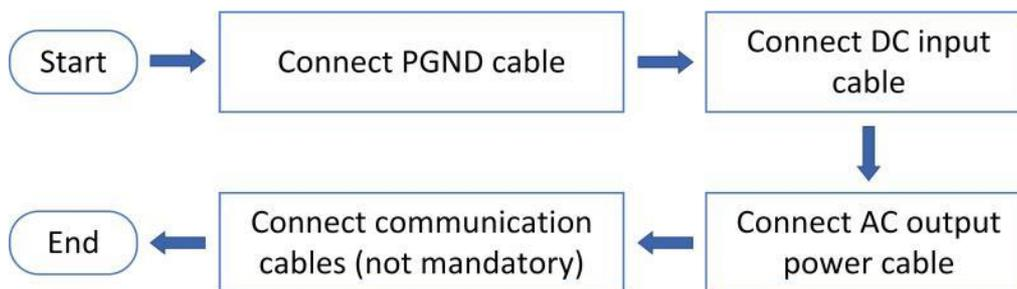
Figure 8 – Steps for connecting the cables
