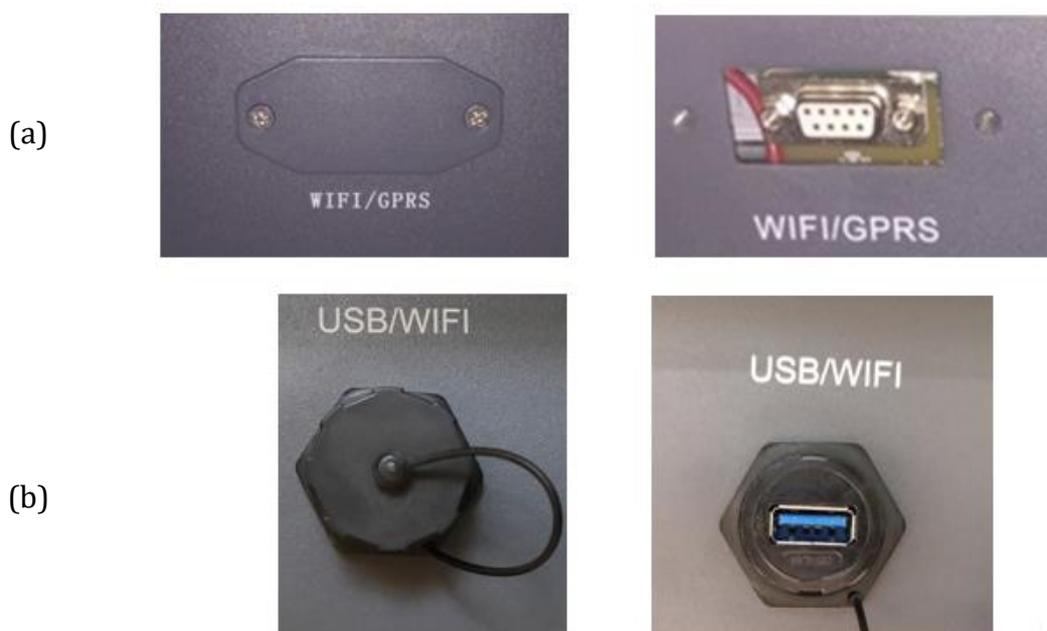
Figure 38 – Port for external Wi-Fi adapter
