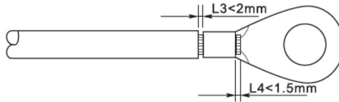
Figure 107 - Preparing the ground cable (2)
