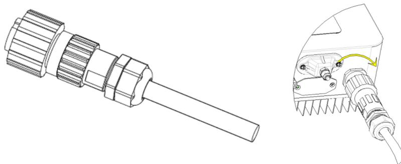
Figure 21 - Connecting the AC output cables (4)
