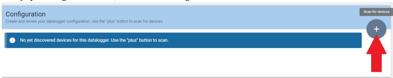
A window will open where you can search for each type of device connected to the Datalogger, after indicating the range of addresses associated with the relative devices.
