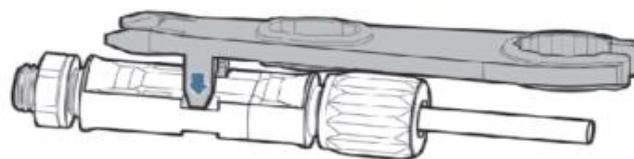
Figure 16 - Removing the DC connector
