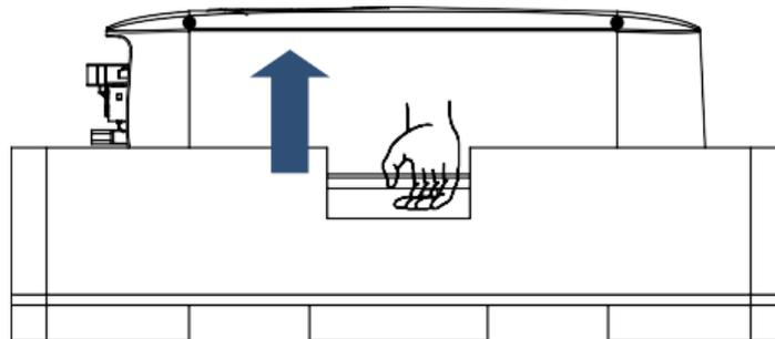
Figure 5 - Removing the polystyrene protections
