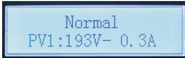
Inverter working status, PV generated power.
