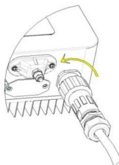
Figure 22 - Disconnecting the AC output cables
