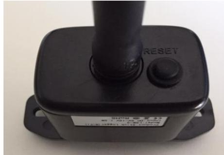
Figure 57 – Reset button on the Wi-Fi adapter
