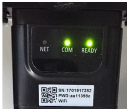
Figure 76 - Irregular communication status between the adapter and remote server
