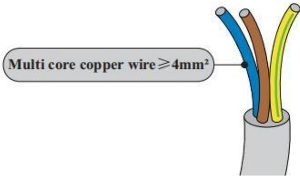
The cross-section of the power line must be sized in order to prevent unwanted disconnections of the inverter from the grid due to high impedance of the cable connecting the inverter to the point of supply. In addition, the AC cable must be correctly sized to ensure that the loss of power on the cable is less than 1% of the rated power and to ensure the proper functioning of the anti-islanding protection. The cable length from the inverter to the grid should not exceed 100 metres.
