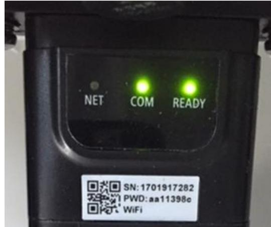
Figure 70 - Irregular communication status between the adapter and remote server
