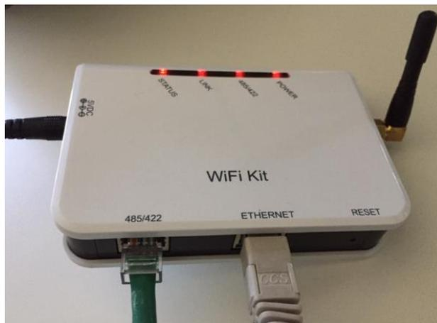
Figure 85 – Ethernet cable connected to the datalogger
