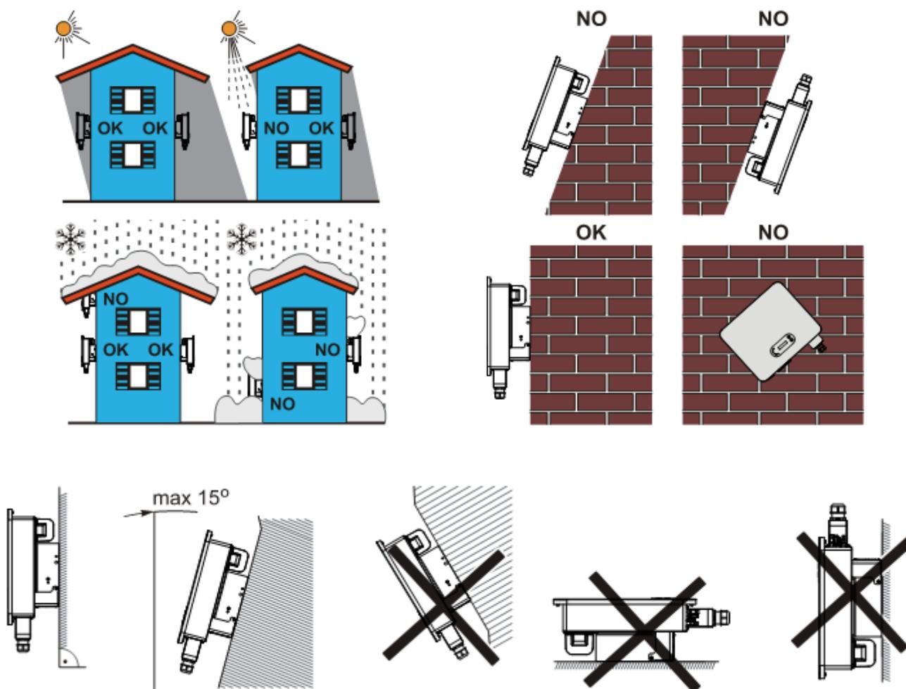
Figure 4 – Requirements for installing a single inverter
