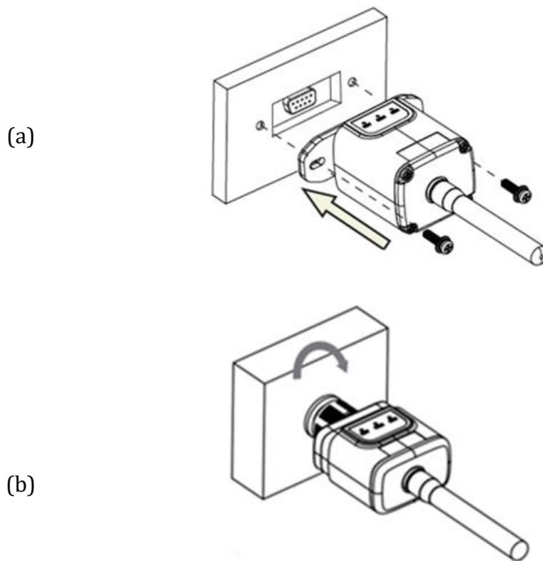
Figure 72 - Inserting and securing the 4G adapter
