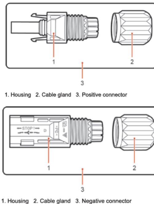
**Figure 12 – Positive (1) and Negative (2) MC4 connectors**
