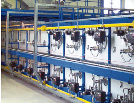
Roller hearth kiln in the ceramics industry
