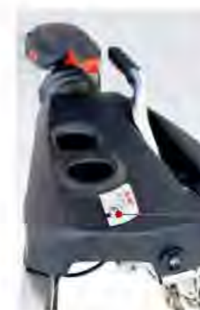
Magnetic switch for activating the transmitter
