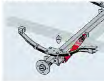
Shock absorber for 750 / 1,500 / 1,800 kg and tandem 3,000 / 3,500 kg
