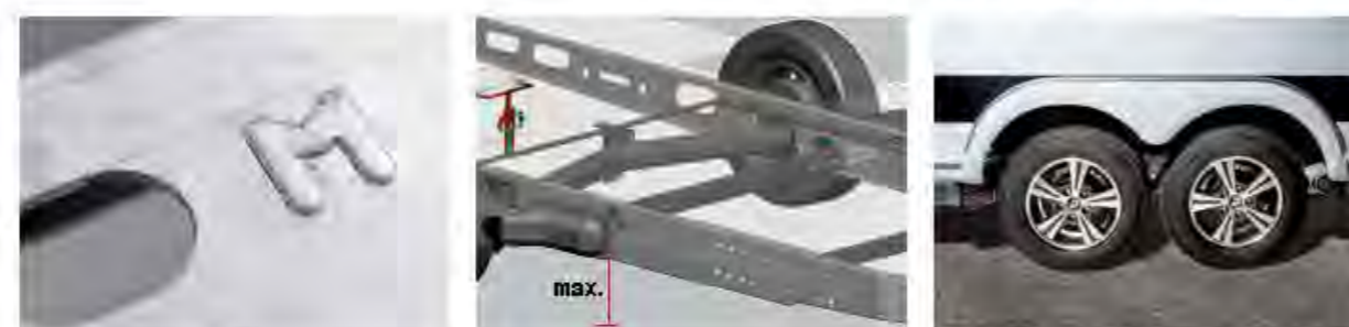
AL-KO chassis with the embossed "M" on the longitudinal frame (SA from model year 2010, TA from model year 2015) have standard mounting holes for the MAMMUT system. The cross member required for stability does not take up any space under the chassis. This ensures maximum ground clearance.
