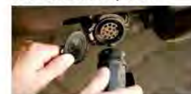
The 13-pin plug establishes the electrical power supply to the car.
