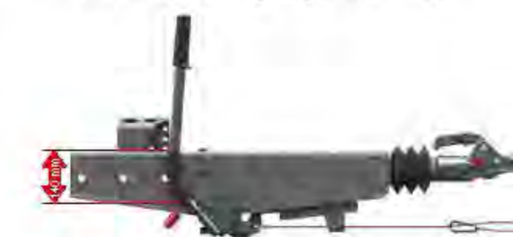
Handbrake lever closed (parking brake backwards, brake optimally set)
