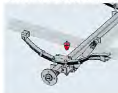
Rubber buffer for 750 / 1,500 / 1,800 kg and tandem 3,000 / 3,500 kg
