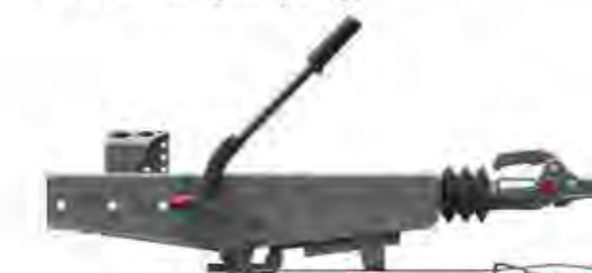
Handbrake lever closed (parking brake forwards)
