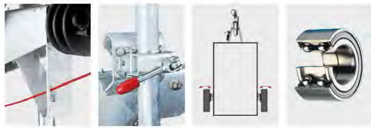
A skid bracket with integrated breakaway cable guide protects the hitch against contamination. The breakaway cable is also guided smoothly, so the emergency brake really does function in an emergency. Jockey wheel flange welded on as standard. Toe-in can be adjusted precisely at the factory for minimum tyre wear. Maintenance-free compact bearing.
