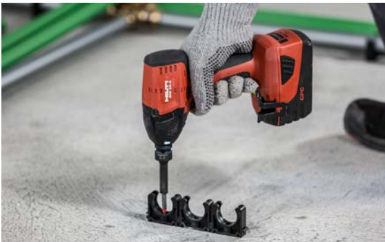
3 Unscrew the HILTI Kwik-Con II+ screw anchor ...
