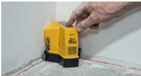
Position inside corner to check for square.
